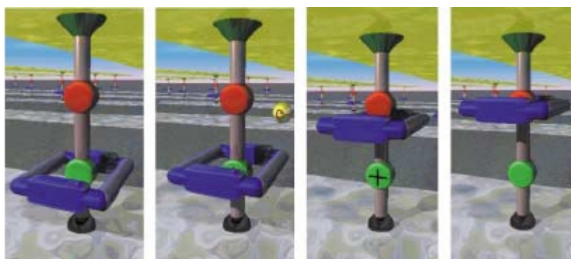
Figure 2.10: Schematic of the amphiphilic rotaxanes in a tunnel junction where the ring (blue) shuttles between the two docking stations. In the beginning, the ring is located at the TTF unit (green), but oxidation leads to coulomb repulsion forcing the ring to translocate to the DNP unit (red). Reduction of the TTF unit first leads to a metastable state before the ring shuttles back to the TTF unit. 50a
